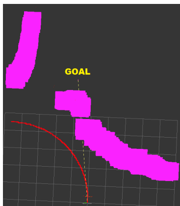
Fig. 6. Visualization of the robot dodging an obstacle.
