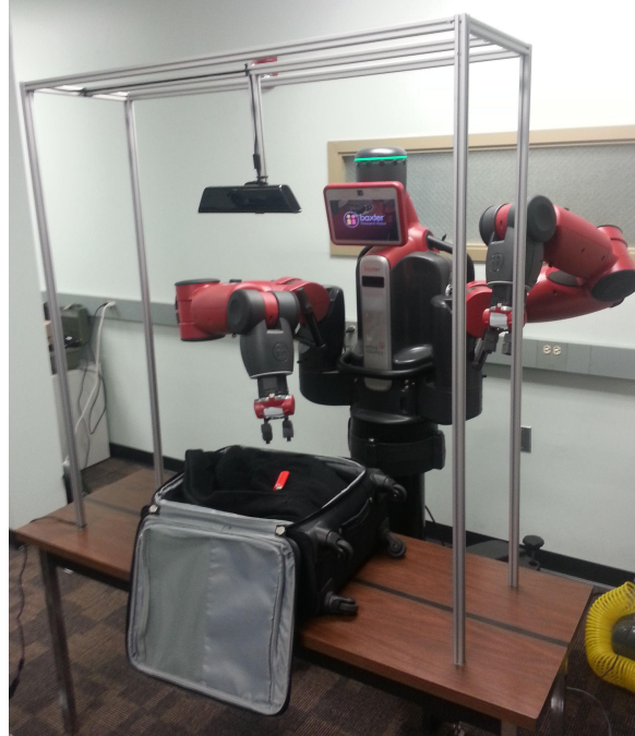
Figure 2. A picture showing Baxter along with the test setup for the case study. Baxter can work in close proximity to humans and utilize an intuitive user interface enabling flexible operations in a variety of scenarios. The robot can be trained and retrained while in the field for performing different tasks.
